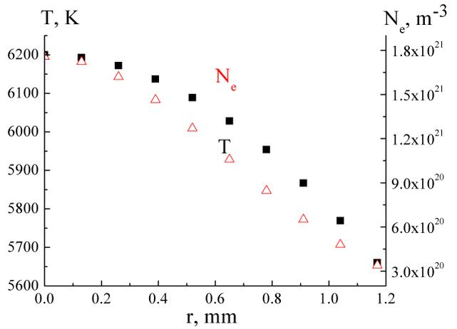
Figure 1. Radial distributions of plasma temperature and electron density of arc discharge between composite Cu–Cr electrodes at current 3.5 A.
