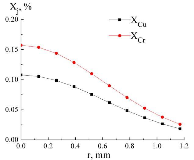
Figure 3. The radial distributions of copper and chromium vapours contents in plasma of electric arc discharge between composite Cu–Cr electrodes at current 3.5 A.
