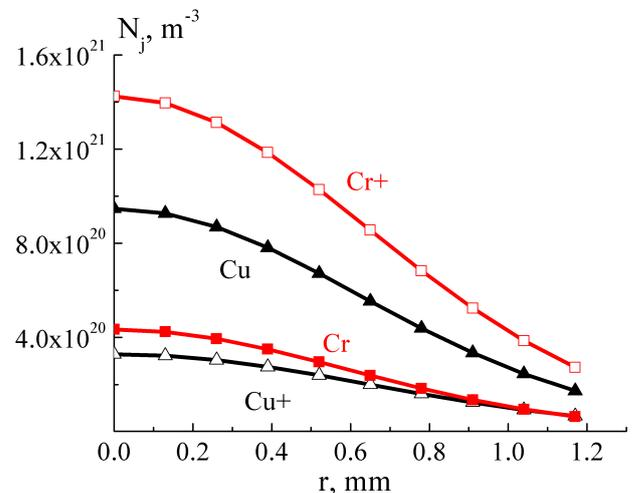
Figure 4. The radial distributions of Cu, Cr atoms and  $Cu^+$ ,  $Cr^+$  ions concentrations.
