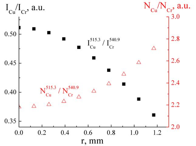
Figure 2. The ratio of the radiation intensity of the spectral lines Cu I 515.3 nm and Cr I 540.9 nm (■). The ratio of concentrations of copper and chromium atoms (△).
