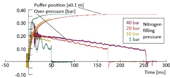
Figure 7. Piston movement and puffer over-pressure as a function of time for all filling pressures (no current). Due to flawed oscilloscope setting, parts of the trace at 10 bar is missing. Due to noise, the piston position for 40 bar was not recorded properly.
