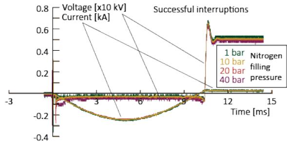
Figure 6. Successful interruptions for different filling pressures. All tests were performed with a charging voltage of 6 kV, resulting in a current peak of 240 A and a TRV first peak of 6.3–6.4 kV.
