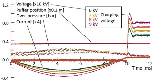
Figure 5. Resulting current and TRV for different charging voltages with 1 bar<sub>abs</sub> nitrogen filling pressure.
