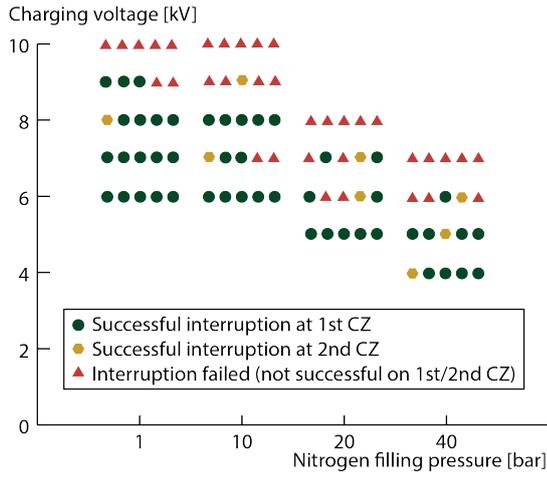
Figure 4. Outcomes of all tests. The coloured symbols (green, yellow and red) represent successful, successful at 2nd half cycle and failed interruption.
