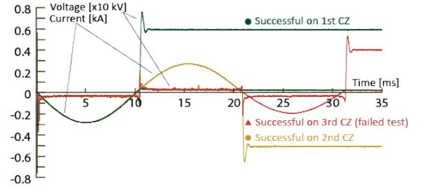
Figure 3. Examples of a successful interruption at the first CZ, at the second CZ, and a failed interruption (interrupted at 3rd CZ).
