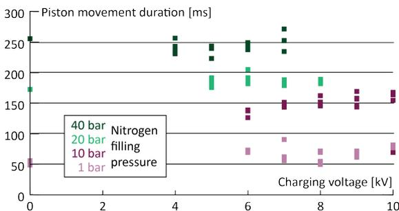
Figure 8. The time from the piston starts moving until it reaches its end point during current interruption tests for all filling pressures and charging voltages.
