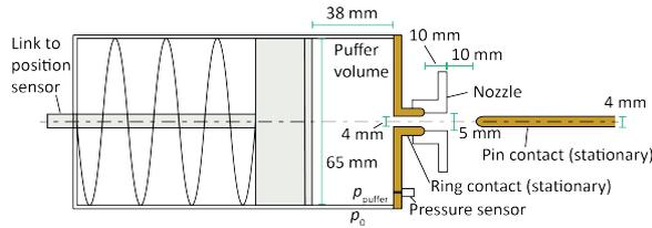
Figure 2. The puffer-type contact configuration. The nozzle was made of polytetrafluoroethylene (PTFE), and the contact material was copper tungsten (CuW, 20/80).
