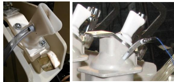
Fig. 2: Pressure sensor tube placements: (a) at the extinguishing nozzle and (b) at the cylinder
