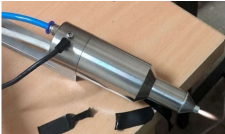
Figure 3. View of the plasma pen in active state and plasma formation.
