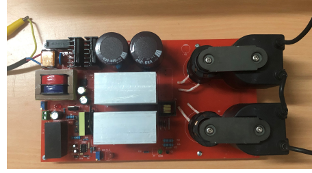
Figure 4. The power supply unit used to create the plasma.
