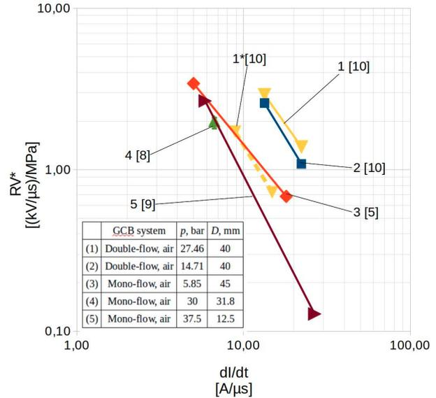
Figure 2. Normalized parameter  $RV^*$  as a function of  $dI/dt$ .
