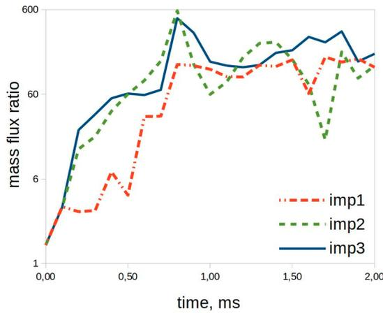
Figure 3. Mass flux ratio  $Q/Q_0$  in zone 1 for different injectors sites (imp1, imp2, imp3).
