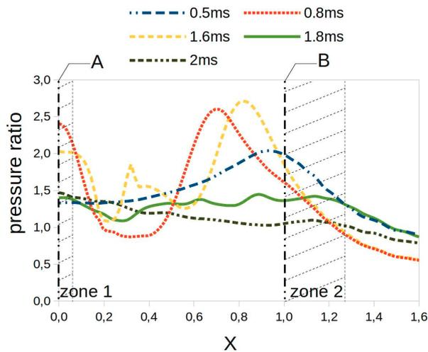
Figure 4. Pressure ratio along OX for various times from injection beginning at imp3.
