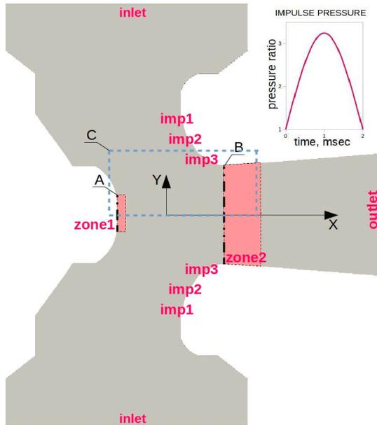
Figure 1. The model of the mono-flow gas blast arc quenching device.
