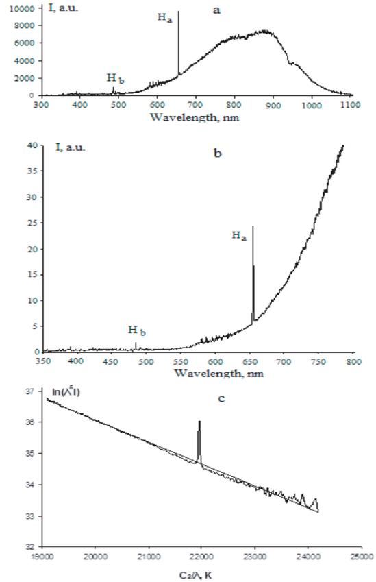
Figure 2. Emission spectrum of the discharge in hydrogen before (a) and after (b) adjustments and in Wynn coordinates (c)
