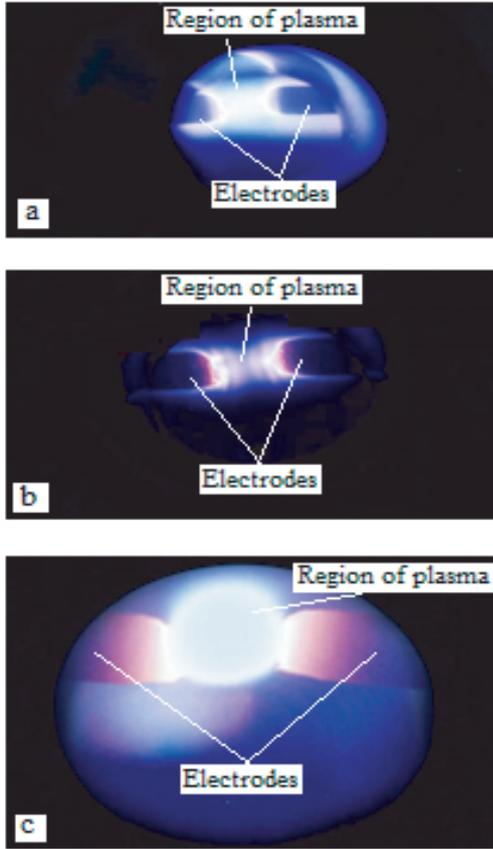
Figure 1. View of gas discharge; a -  $P=100$  Torr  $H_2$ , b - 760 Torr  $H_2$ , c - 760 Torr  $H_2 + SiCl_4$ .
