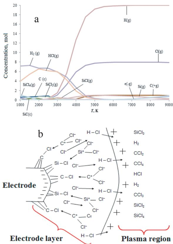
Figure 4. a - Temperature dependence of composition of the main conversion products at 1 atm. pressure for  $\text{SiCl}_4 + \text{CCl}_4 + 10\text{H}_2$  system, b - Mechanism of deposition of SiC.
