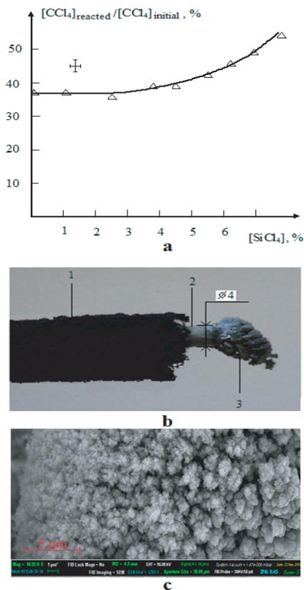
Figure 3. a - Dependence of conversion degree of CCl<sub>4</sub> on the content of SiCl<sub>4</sub> in the initial mixture; b - View of electrode: 1 - nozzle, 2 - silicon electrode, 3 - deposited SiC and c - morphology of deposited SiC.
