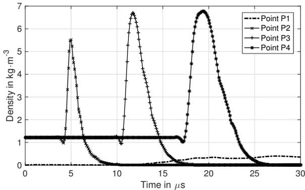
Figure 6. Density of the plasma in dependence of the time for the selected points
