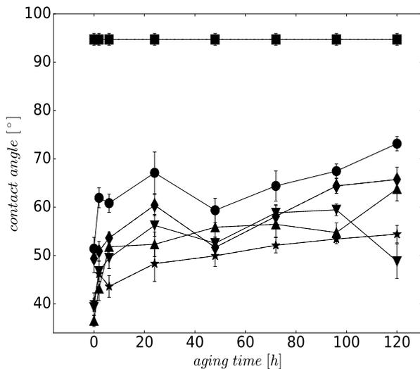
Figure 4. The water contact angle for ABS treated on the DCSBD with different exposure times, (●) 1 s, (◆) 3 s, (▲) 5 s, (▼) 10 s, (★) 30 s, (■) reference
