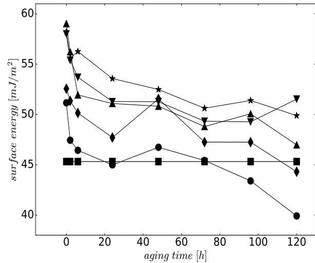
Figure 5. The surface energy for ABS treated on the DCSBD with different exposure times, (●) 1 s, (◆) 3 s, (▲) 5 s, (▼) 10 s, (★) 30 s, (■) reference
