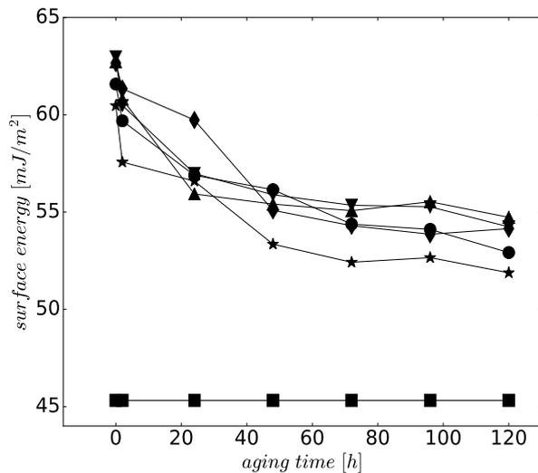
Figure 8. The surface energy for ABS treated on the Gliding arc with different exposure times, (●) 1 s, (◆) 3 s, (▲) 5 s, (▼) 10 s, (★) 30 s, (■) reference
