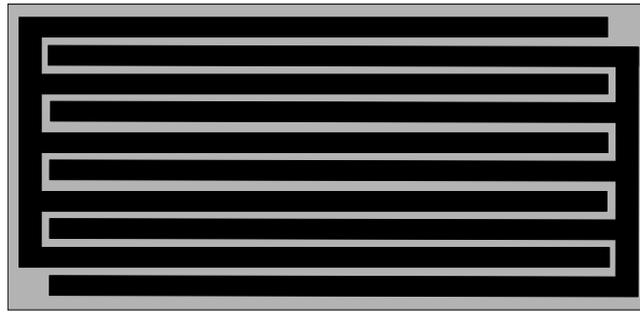
Figure 1. The coplanar arrangement of the electrodes
