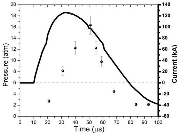
Fig.3: Plasma pressure (dots, left scale) and discharge current (solid line) vs. time for  $U_0=4.5$  kV
