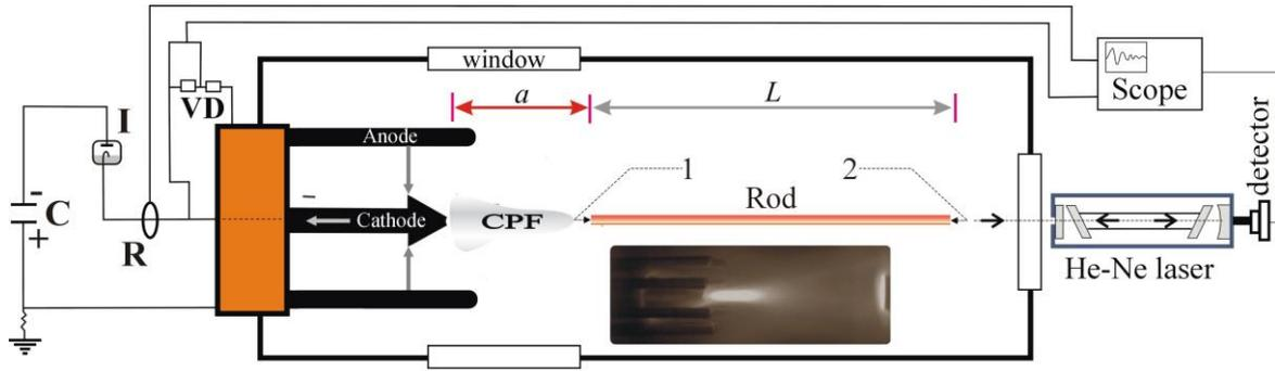
Fig.1: Experimental setup: C—capacitor, I—ignitron, R—Rogowski coil, VD—voltage divider
