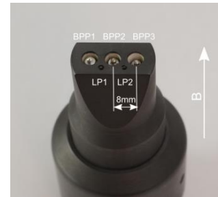
Fig.1: Picture of the probe head exploited in the described experiments. As it is seen, the shield of the probe head is made of graphite to survive the heat flux.
