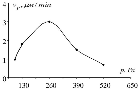
Fig.3: Dependence of photoresist removal rate on the pressure of oxygen in the discharge chamber
