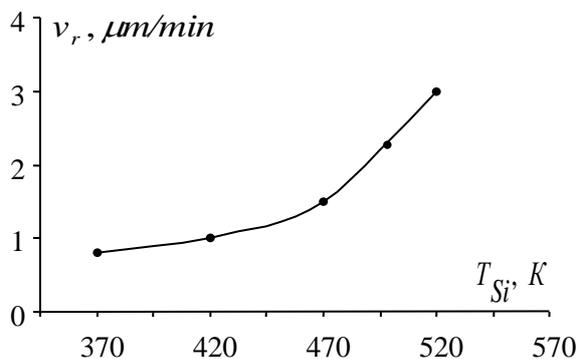
Fig. 2: Dependence of photoresist removal rate on the substrate temperature
