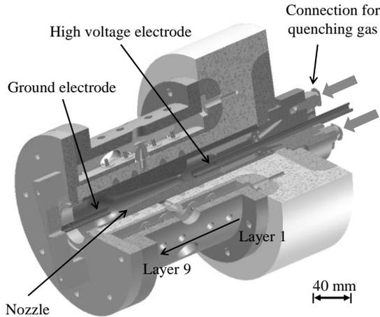
Fig. 1: Sketch of the circuit breaker model of the contactless measurement system
