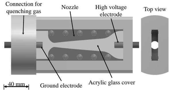
Fig. 2: Sketch of the optical circuit breaker model
