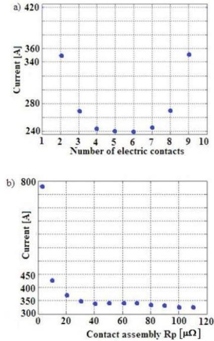
Fig. 4: a) Syneresis of the current in the flat contact assembly at  $R_p = 5 \mu\Omega$ , b) relation of the value of the floating electricity in extreme fuse of contact assembly ad valorem of contact resistance
