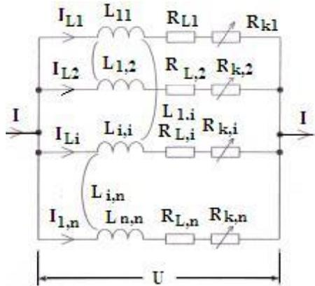
Fig. 3: Schematic diagram of the inspected contact assembly,  $i$  - total electricity,  $I_{L1}$ ,  $I_{Li}$ ,  $I_{Ln}$  - currents in individual zones of power rail,  $L_{1,1}$ ,  $L_{1,2}$ ,  $L_{1,i}$ ,  $L_{i,i}$ ,  $L_{i,n}$  - inductance own and mutual,  $R_{L1}$  - resistance of the electric contact,  $R_{ki}$  - resistance of the contact assembly
