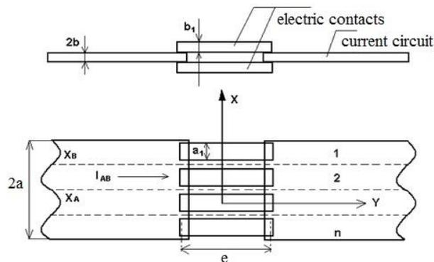
Fig. 1: Outline of arranging of electric contacts in the contact assembly, 1, 2, ... n - of electric contacts, 2a, 2b - dimensions of joints, a<sub>1</sub>, b<sub>1</sub> - dimensions of electric contacts
