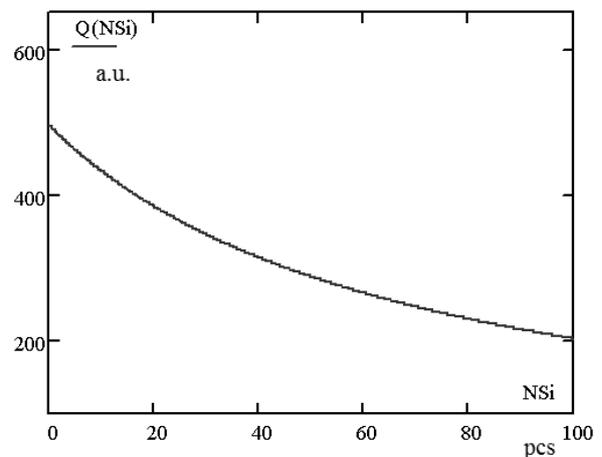
Fig.4: Dependence of total quality factor of the cavity resonator partially filled with plasma  $Q$  on the number of silicon wafers loaded into it
