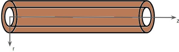
Figure 2. Geometry used for the 3D heat conduction study. Only the solid region (in brown) is modelled. The inside radius is  $R_{int}$ , the external radius is  $R_{ext}$ , and the length of the cylinder is  $H$ .
