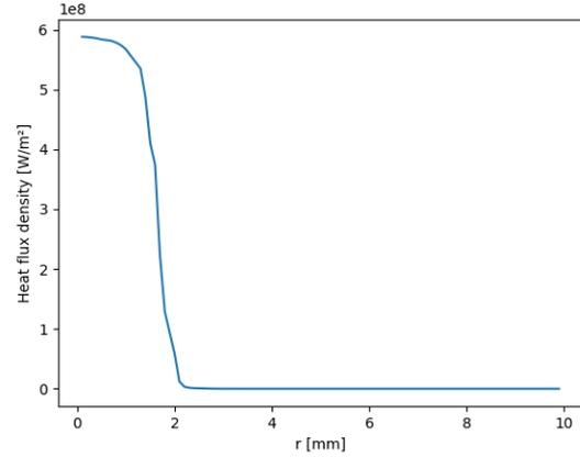
Figure 3. Cathodic heat flux profile for an electric arc in air, with current intensity  $I = 260 \text{ A}$  and  $\beta = 40$
