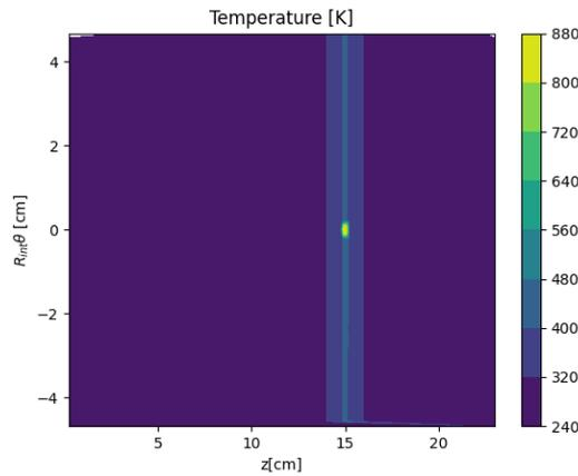
Figure 5. Temperature field on the inner cathode surface after 1 s of heating.
