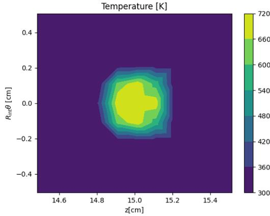
Figure 4. Temperature field on the internal surface of the cathode after  $10 \mu\text{s}$ . This temperature spot moves on the cathode surface in agreement with the flux spot.
