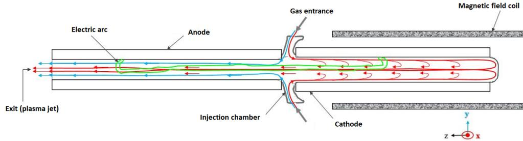
Figure 1. Sketch of the hollow cathode plasma torch working principle
