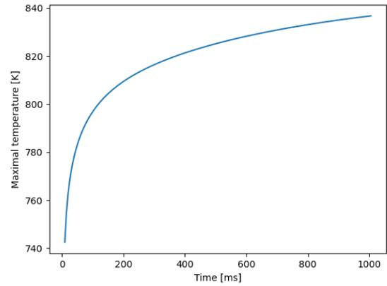
Figure 6. Evolution of the maximal temperature reached on the inner cathode surface for  $h = 35000 \text{ W.m}^{-2}.\text{K}^{-1}$ .
