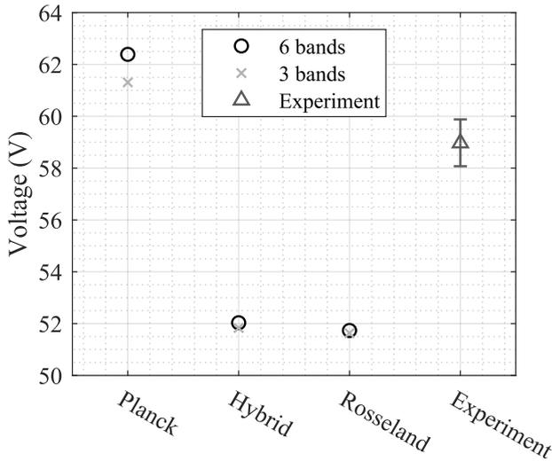
Figure 3. Mean arc voltage of three- and six-band selection for different averaging methods. The experimental mean, as well as the minimum and maximum value of the test series from [8] are shown for comparison.
