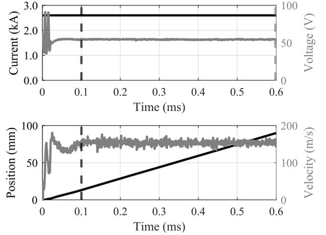
Figure 2. Simulation results of arc current, voltage, position, and velocity of exemplary simulation with six-band hybrid MAC.
