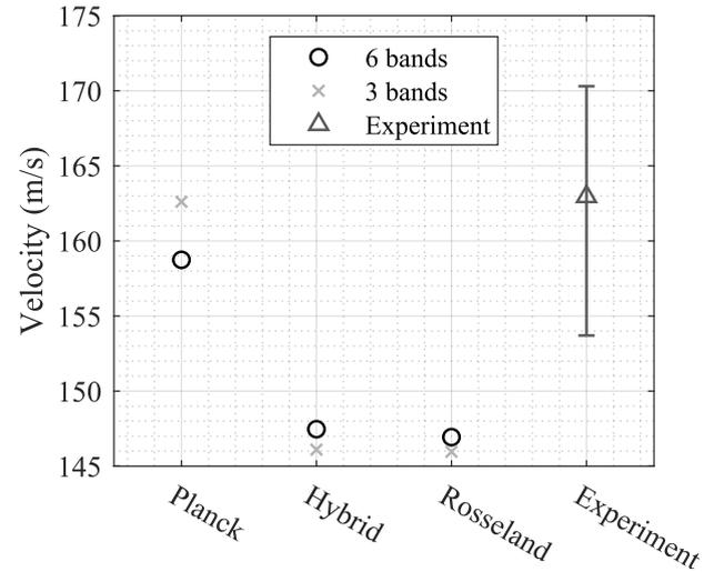
Figure 4. Mean arc velocity of three- and six-band selection for different averaging methods. The experimental mean, as well as the minimum and maximum value of the test series from [8] are shown for comparison.
