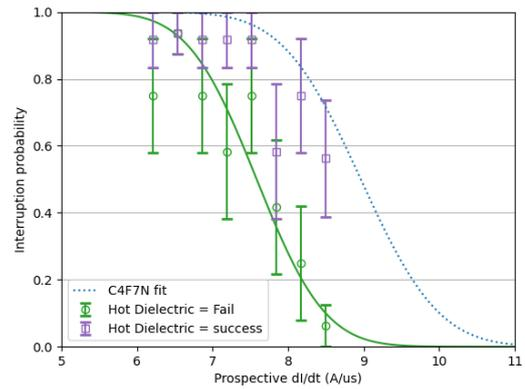
Figure 7. Influence of "hot dielectric" breakdowns treated as failures (green) or successes (purple) to determine thermal interruption performance of CO<sub>2</sub>. The fit of CO<sub>2</sub>/C<sub>4</sub>F<sub>7</sub>N is plotted as reference.
