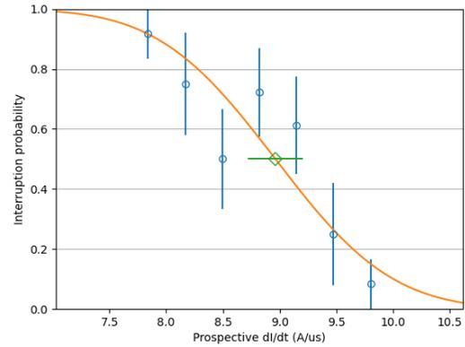
Figure 2. Thermal interruption limit determination of  $\text{CO}_2/\text{C}_4\text{F}_7\text{N}$ . Blue circles and lines - the probability of success from the binomial distribution, orange line - cumulative function fit, green diamond - interruption limit with two sigma uncertainty interval.
