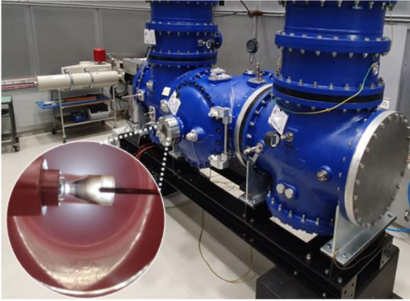
Figure 1. Experimental setup of Puffer CB
