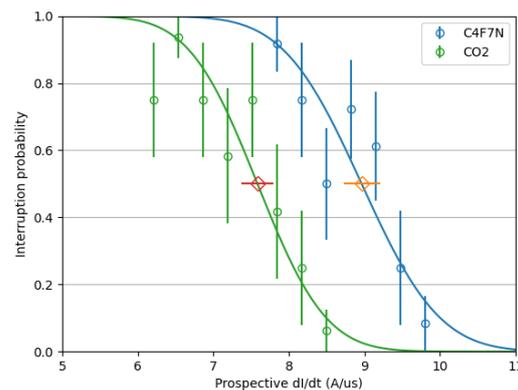
Figure 4. Thermal interruption limit for  $\text{CO}_2$  and  $\text{CO}_2/\text{C}_4\text{F}_7\text{N}$
