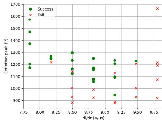
Figure 3. Extinction peak in function of  $di/dt$  measured in  $\text{CO}_2/\text{C}_4\text{F}_7\text{N}$  gas mixture.
