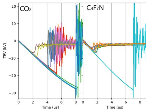
Figure 6. Few TRV measurements in case of failures in CO<sub>2</sub> left and in CO<sub>2</sub>/C<sub>4</sub>F<sub>7</sub>N right
