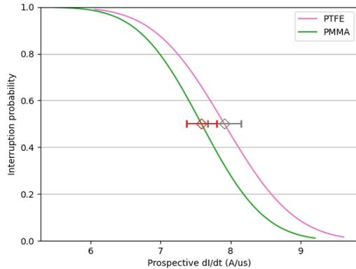
Figure 8. Thermal interruption performance of  $\text{CO}_2$  with PMMA and PTFE nozzle
