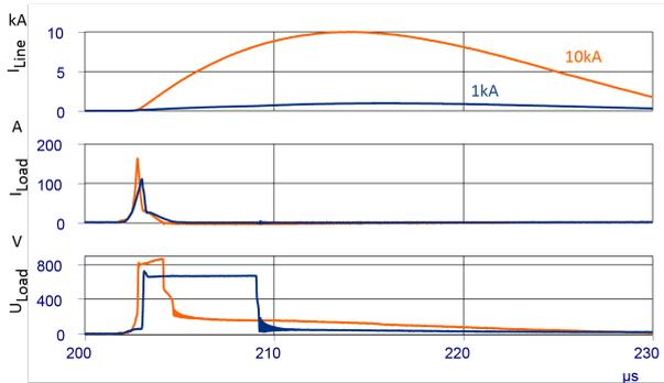
Figure 4. Behaviour of the arrangement in case of transient currents 1 kA (blue) and 10 kA (orange) 8/20 μs top - transient impulse line current; middle - transient impulse load current after switch; bottom - load voltage
