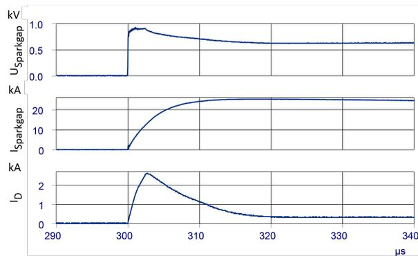
Figure 7. Behaviour of common triggerable spark gap during a lightning current of 25 kA 10/350  $\mu$ s top - voltage spark gap and consumer, middle - impulse current spark gap, bottom - impulse current load / consumer in case of a varistor (S20K275) within the consumer
