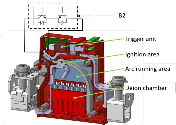
Figure 5. Spark gap with trigger unit and additional actuation by B2
