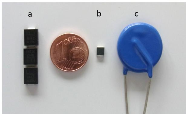
Figure 8. Picture of suitable overvoltage protective components for use as secondary protection D or within consumer C by use of the tested arrangement a - suppressor diodes; b - SMD varistor; c - normal varistor S20K275
