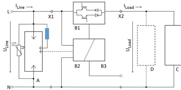
Figure 2. Principle of the recommended protective arrangement A - triggerable spark gap; B1 - switch; B2 - monitoring unit; B3 - control device; C - consumer; D - secondary protection
