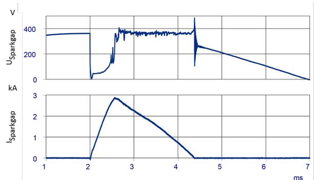
Figure 6. Arc extinction at a mains voltage of 230 V AC at a prospective short-circuit current of 25 kA
