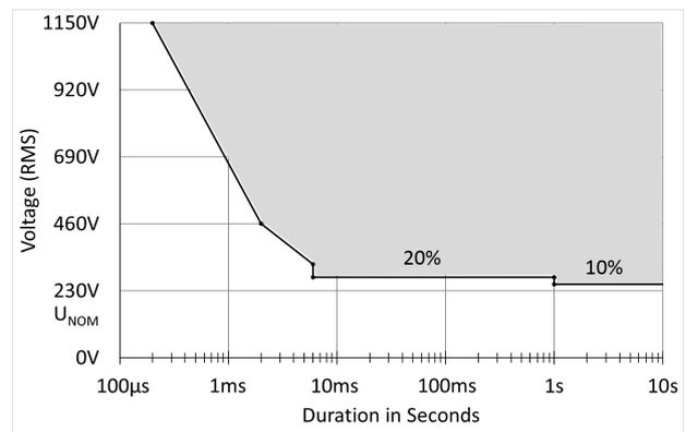
Figure 1. Voltage tolerance curve proper for 230 Volt AC equipment
