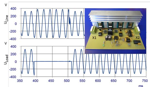
Figure 3. Behaviour of the arrangement in case of line frequency overvoltage top - line voltage; bottom - load voltage, picture of the switch B1 with control and monitoring unit
