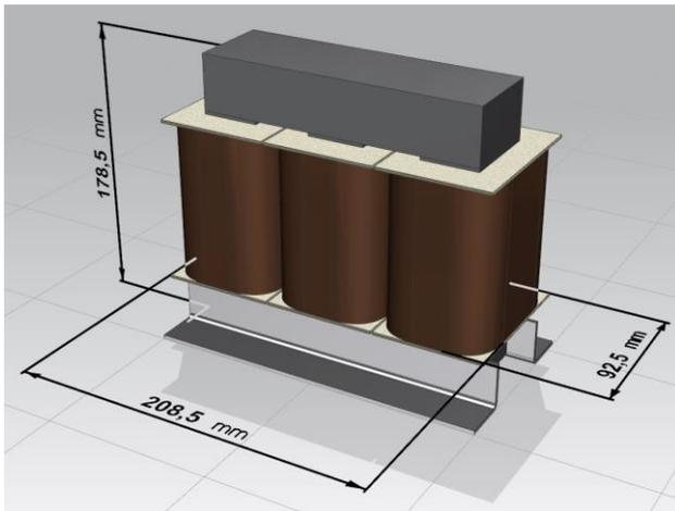
Fig. 2. 3D CAD model of sinus filter.
