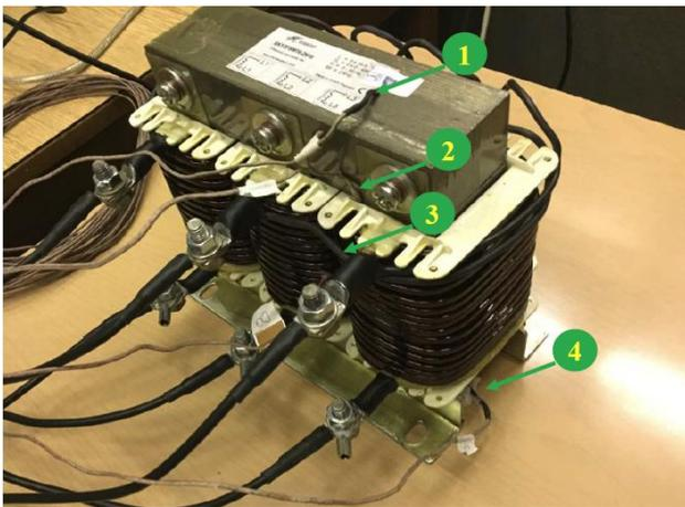
Fig. 4. Sinus filter SKY3FSM16-2kHz with thermocouples.
