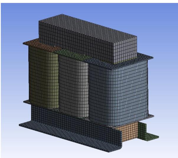
Fig. 3. Mesh of sinus filter 3D model.
