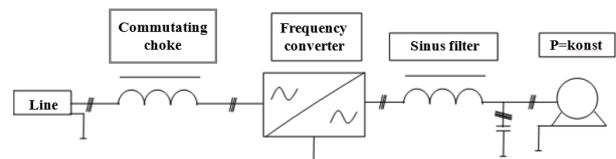
Fig. 1. Schematic wiring description of sinus filter.
