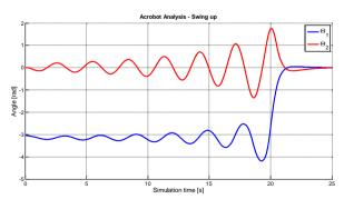
Fig. 10. Swing-up and subsequent stabilization of the Acrobot in the upright position.
