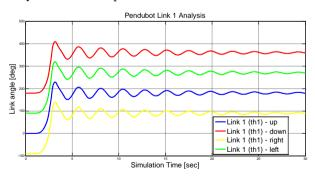
Fig. 7. Simulations of a Pendubot first link – effect of the changing reference positions.
