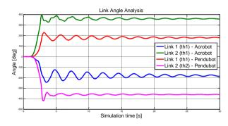
Fig. 6. Open-loop behavior of Acrobot and Pendubot.
