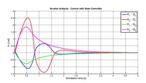
Fig. 8. Stabilization of the Acrobot in the upright unstable position.
