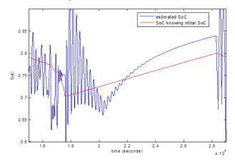
Fig. 7. Comparison of SoC with the knowledge of initial SoC and estimated SoC.
