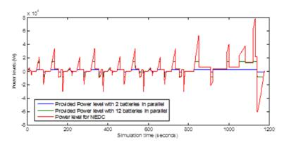
Fig. 13. Different power profiles associated with change in number of batteries in parallel.
