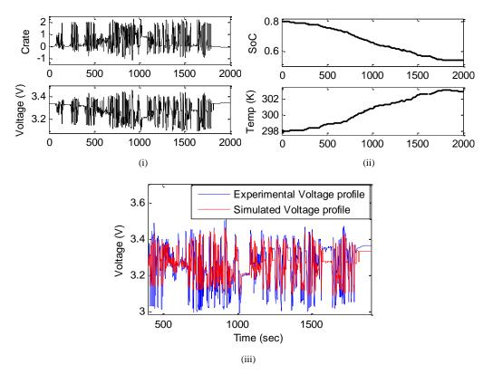
Fig. 5. (i-ii) Current, voltage, SoC and temperature profile. (iii) Real and simulated voltage profiles.
