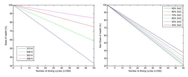
Fig. 4. SoH calculation different initial SoC and temperature.
