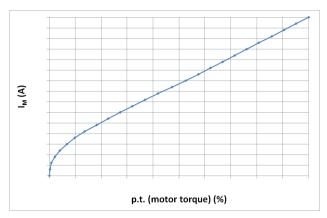
Fig. 6. Traction motor armature current - torque curve.
