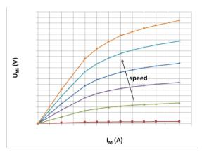
Fig. 7. Induced voltage of the traction motor for full excitation.
