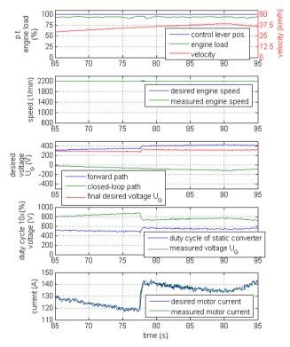
Fig. 10. Field weakening of traction motors.
