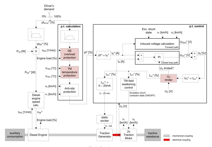
Fig. 4. Control structure.
