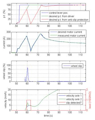
Fig. 5. Anti-slip protection.
