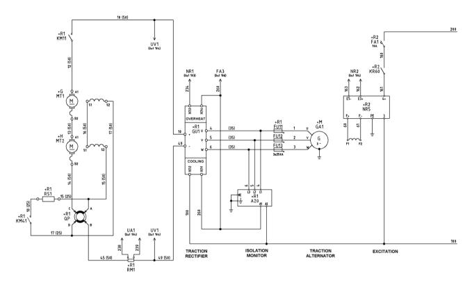
Fig. 2. Traction drive electrical circuit [8].
