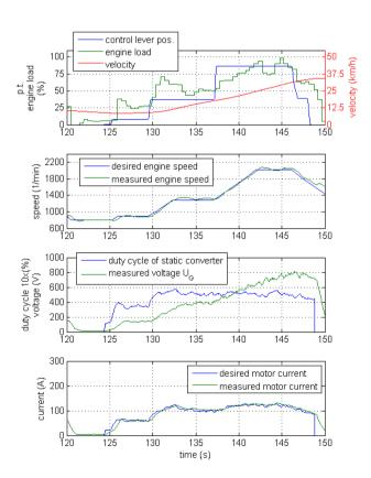
Fig. 9. Motor current control - acceleration at 100 % p.t.
