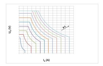
Fig. 3. Load curve of the traction generator.
