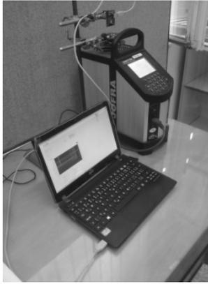
Fig. 5. Calibration - assembly of measuring system during calibration.
