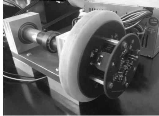
Fig. 3. System for data transport – rotating parts.
