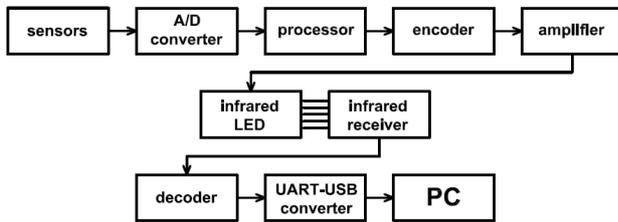
Fig. 2. The block diagram of the measuring system.
