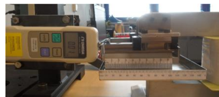
Fig. 9. Apparatus for measuring the static force characteristics of the actuator.
