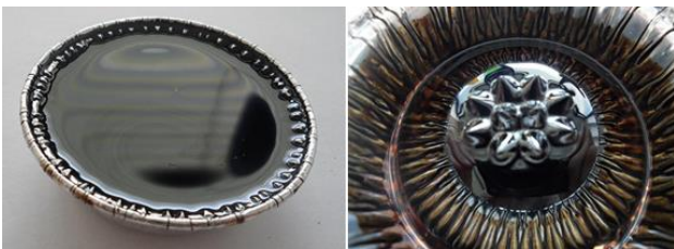
Fig. 1. Ferrofluid EFH-1 without and with applied magnetic field.
