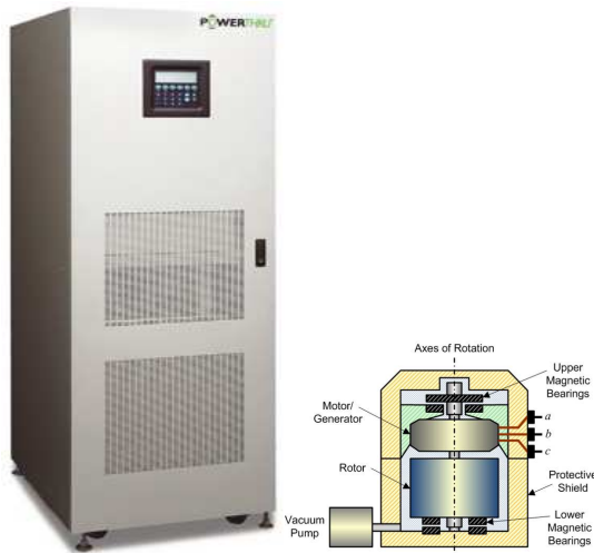
Fig. 1. UPS system working with FES, http://www.power-thru.com/
