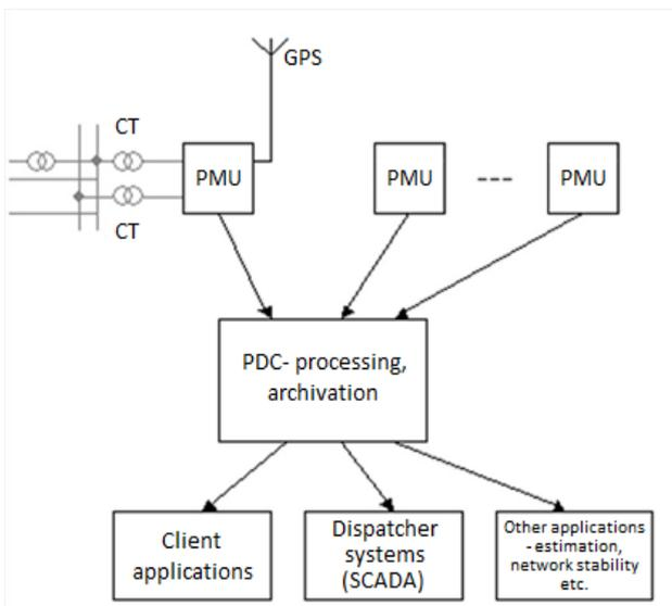
Fig. 2. Structural diagram of synchrophasor system
