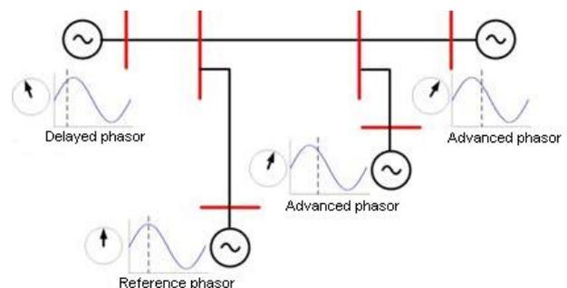
Fig. 2. Snap of relative phasors with reference measurement
