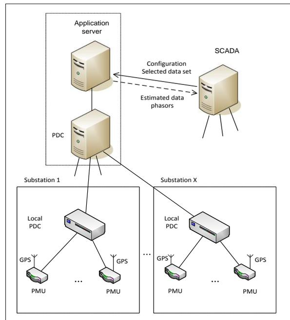
Fig. 3. System with the local PDC
