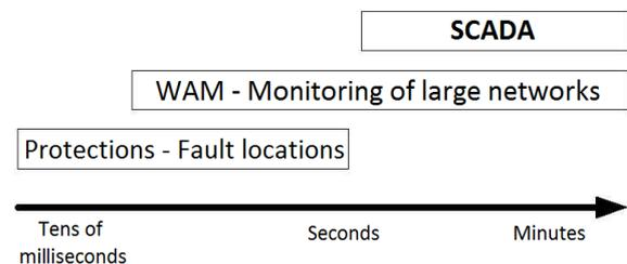
Fig. 6. Requirements for the measurement/communication speed for various systems
