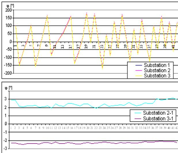
Fig. 1. Sample of synchronous and relative phasors (Substation 1 is selected as reference measurement)
