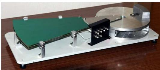
Fig. 11. Capacitive sensor of the angle of rotation
