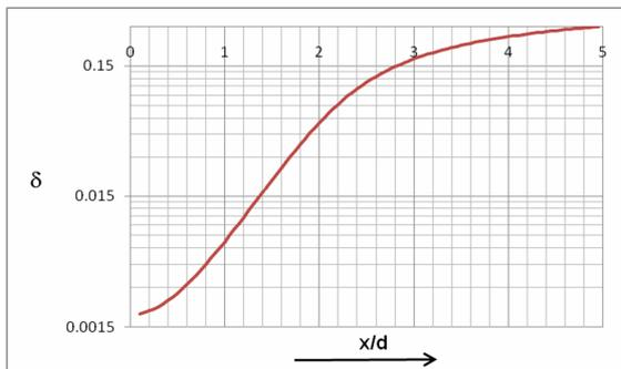
Fig. 9 b) Linearity error, differential sensor,  $x_0=2d$
