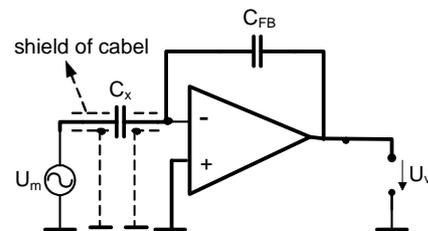
Fig. 12. Elimination of parasitic capacitances of leads.
