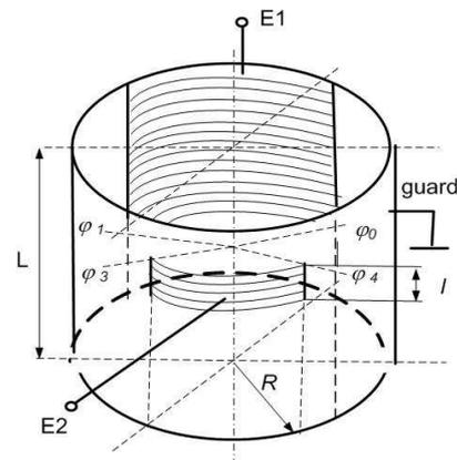
Fig. 4 Cylindrical sensor
