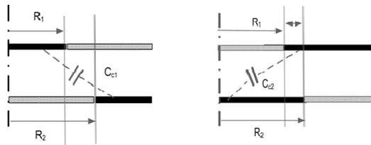
Fig. 6. Cross-capacitances of circular electrodes
