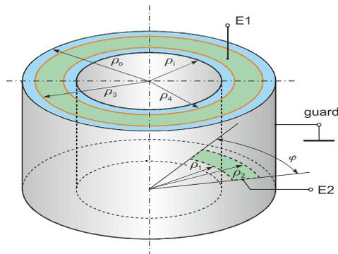
Fig.3. The archetype of the torus shaped capacitive sensor
