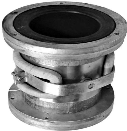
Fig. 3. Photograph of flow meter inner part.
