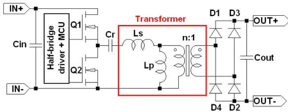
Fig. 3. The principal schema of proposed LLC converter
