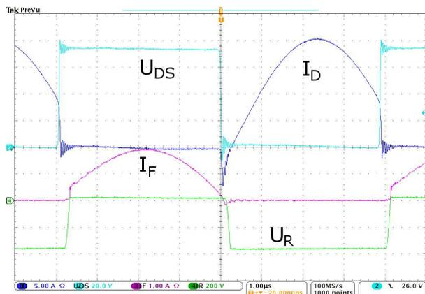
Fig. 7. Measured waveforms of currents and voltages on the primary MOSFET and the rectifier diode.
