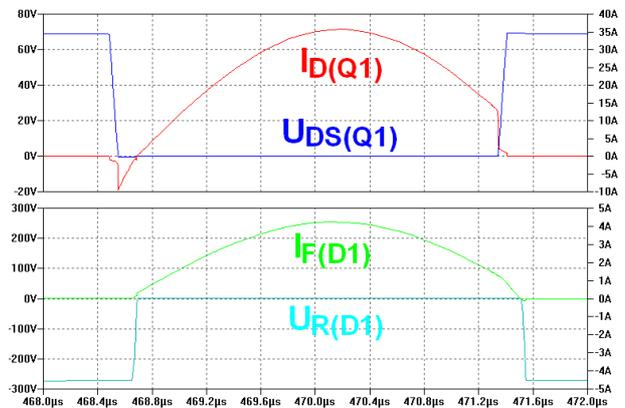
Fig. 6. Simulated waveforms of voltages and currents on switch Q1 and diode D1.
