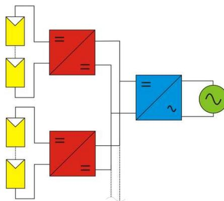
Fig. 2. Topology of converter for photovoltaic system connected to grid
