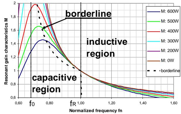
Fig. 4. Voltage gain curves of the resonant tank.
