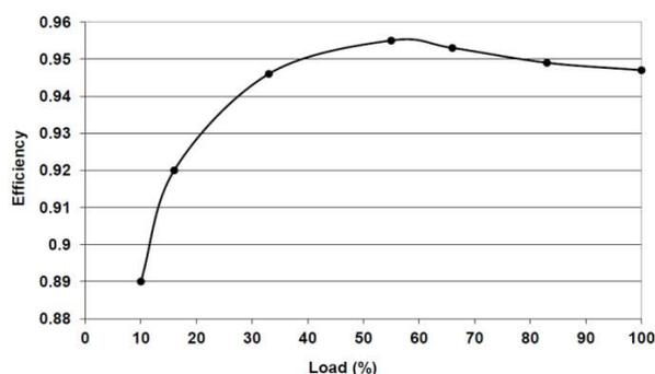
Fig. 8. Measured efficiency of the converter.
