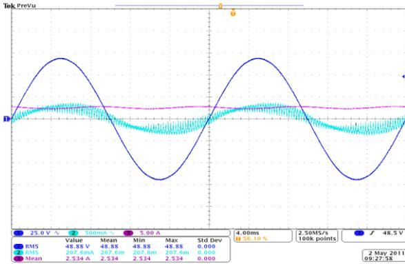
Figure 9a. Sinusoidal supply voltage, steady-state, without compensation,  $I_d=2.5$  A,  $\phi = 0^\circ$ ,  $V_s = 50$  V<sub>rms</sub>/50 Hz (Ch1- $v_s$ , Ch2- $i_s$ , Ch3- $I_d$ )
