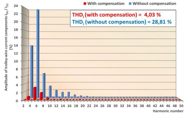
Figure 14. Comparison of harmonic analysis of trolley-wire current from Fig. 10a (without compensation) and Fig. 10b (with compensation)
