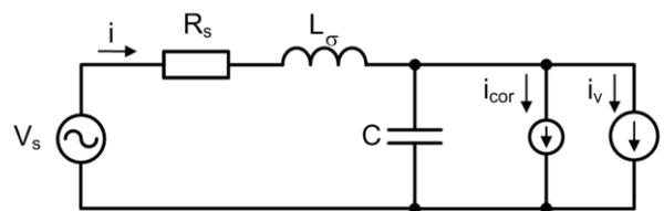
Figure 2. Simplified circuit of the active harmonic elimination applied to the active current-source rectifier
