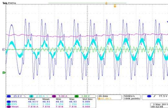
Figure 15. Step change of  $V_s$  from sinwave to waveform 2, with compensation.,  $I_d = 8A$ ,  $\varphi = 0^\circ$ ,  $V_s = 50 V_{rms}/50 Hz$  (Ch1- $v_s$ , Ch2- $i_s$ , Ch3- $I_{dt}$ , Ch4 ( $i_{cor}$ )-0.5 A/DIV)
