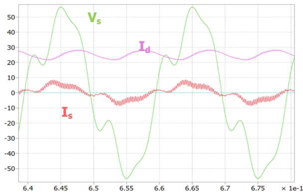
Figure 4a. Waveform 1, steady-state, without compensation,  $I_d=2,5$  A,  $\varphi=0^\circ$ ,  $V_s=50$  V<sub>rms</sub>/50 Hz ( $V_s=10$  V/DIV,  $I_s=1$  A/DIV,  $I_d=1$  A/DIV)
