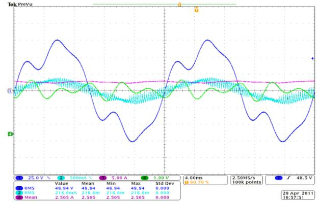
Figure 7b. Waveform 1, steady-state, with compensation,  $I_d = 2.5$  A,  $\varphi = 0^\circ$ ,  $V_s = 50$  V<sub>rms</sub>/50 Hz (Ch1-v<sub>s</sub>, Ch2-i<sub>s</sub>, Ch3-I<sub>d</sub>, Ch4 ( $i_{cor}$ )-0.5A/DIV)
