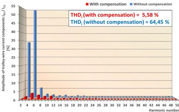
Figure 11. Comparison of harmonic analysis of trolley-wire current from Fig. 7a (without compensation) and Fig. 7b (with compensation)
