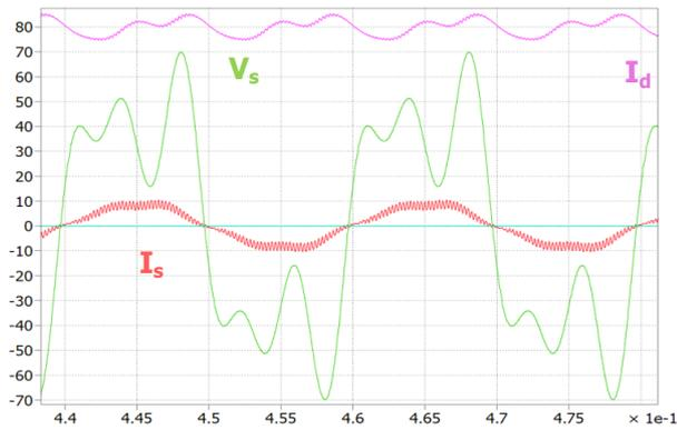
Figure 6a. Waveform 2, steady-state, without compensation,  $I_d=8$  A,  $\varphi=0^\circ$ ,  $V_s=50$  V<sub>rms</sub>/50 Hz ( $V_s=10$  V/DIV,  $I_s=5$  A/DIV,  $I_d=1$  A/DIV)
