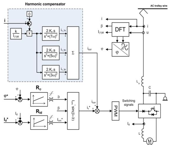
Figure 1. Proposed control strategy with the phase shift controller and active correction of the trolley-wire current waveform
