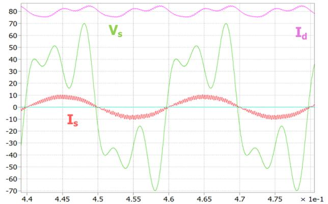
Figure 6b. Waveform 2, steady-state, with compensation,  $I_d=8$  A,  $\varphi=0^\circ$ ,  $V_s=50$  V<sub>rms</sub>/50 Hz ( $V_s=10$  V/DIV,  $I_s=5$  A/DIV,  $I_d=1$  A/DIV)
