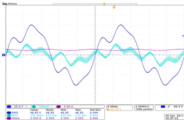
Figure 7a. Waveform 1, steady-state, without compensation,  $I_d = 2.5$  A,  $\varphi = 0^\circ$ ,  $V_s = 50$  V<sub>rms</sub>/50 Hz (Ch1-v<sub>s</sub>, Ch2-i<sub>s</sub>, Ch3-I<sub>d</sub>)
