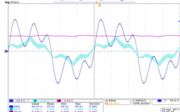
Figure 10a. Waveform 2, steady-state, without compensation,  $I_d=8$  A,  $\phi = 0^\circ$ ,  $V_s = 50$  V<sub>rms</sub>/50 Hz (Ch1- $v_s$ , Ch2- $i_s$ , Ch3- $I_d$ )
