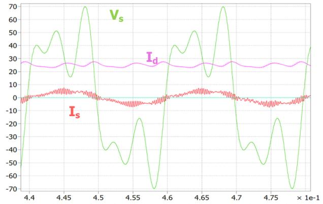
Figure 5b. Waveform 2, steady-state, with compensation,  $I_d=2,5$  A,  $\varphi=0^\circ$ ,  $V_s=50$  V<sub>rms</sub>/50 Hz ( $V_s=10$  V/DIV,  $I_s=1$  A/DIV,  $I_d=1$  A/DIV)
