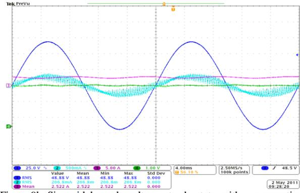
Figure 9b. Sinusoidal supply voltage, steady-state, with compensation,  $I_d=2.5$  A,  $\phi = 0^\circ$ ,  $V_s = 50$  V<sub>rms</sub>/50 Hz (Ch1- $v_s$ , Ch2- $i_s$ , Ch3- $I_d$ , Ch4 ( $i_{cor}$ )-0.5A/DIV)
