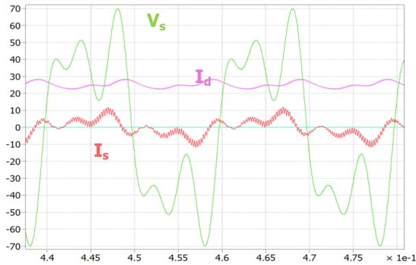
Figure 5a. Waveform 2, steady-state, without compensation,  $I_d=2,5$  A,  $\varphi=0^\circ$ ,  $V_s=50$  V<sub>rms</sub>/50 Hz ( $V_s=10$  V/DIV,  $I_s=1$  A/DIV,  $I_d=1$  A/DIV)
