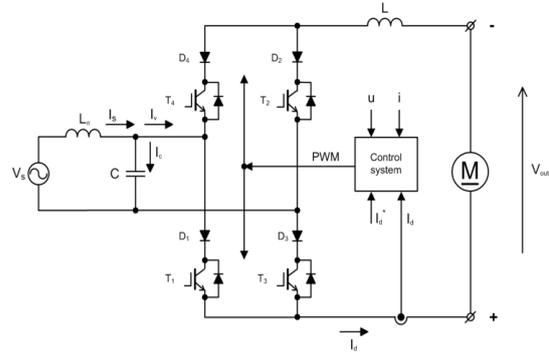
Figure 1. Power circuit of single-phase active current-source rectifier
