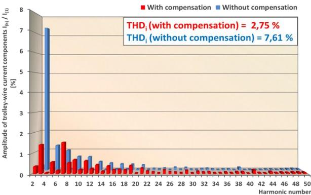
Figure 13. Comparison of harmonic analysis of trolley-wire current from Fig. 9a (without compensation) and Fig. 9b (with compensation)
