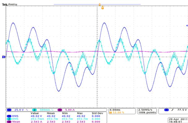
Figure 8a. Waveform 2, steady-state, without compensation,  $I_d = 2.5$  A,  $\varphi = 0^\circ$ ,  $V_s = 50$  V<sub>rms</sub>/50 Hz (Ch1-v<sub>s</sub>, Ch2-i<sub>s</sub>, Ch3-I<sub>d</sub>)
