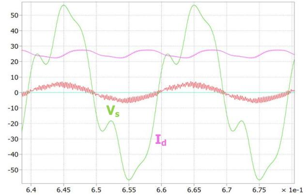
Figure 4b. Waveform 1, steady-state, with compensation,  $I_d=2,5$  A,  $\varphi=0^\circ$ ,  $V_s=50$  V<sub>rms</sub>/50 Hz ( $V_s=10$  V/DIV,  $I_s=1$  A/DIV,  $I_d=1$  A/DIV)
