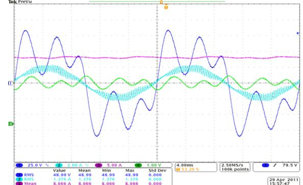
Figure 10b. Waveform 2, steady-state, with compensation,  $I_d=8$  A,  $\phi = 0^\circ$ ,  $V_s = 50$  V<sub>rms</sub>/50 Hz (Ch1- $v_s$ , Ch2- $i_s$ , Ch3- $I_d$ , Ch4 ( $i_{cor}$ )-0.5 A/DIV)
