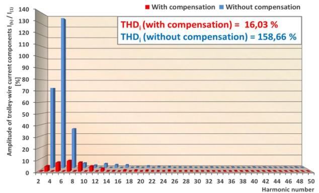
Figure 12. Comparison of harmonic analysis of trolley-wire current from Fig. 8a (without compensation) and Fig. 8b (with compensation)
