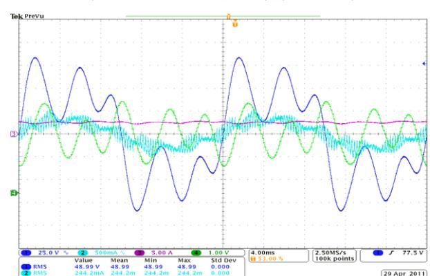
Figure 8b. Waveform 2, steady-state, with compensation,  $I_d = 2.5$  A,  $\varphi = 0^\circ$ ,  $V_s = 50$  V<sub>rms</sub>/50 Hz (Ch1-v<sub>s</sub>, Ch2-i<sub>s</sub>, Ch3-I<sub>d</sub>, Ch4 ( $i_{cor}$ )-0.5 A/DIV)
