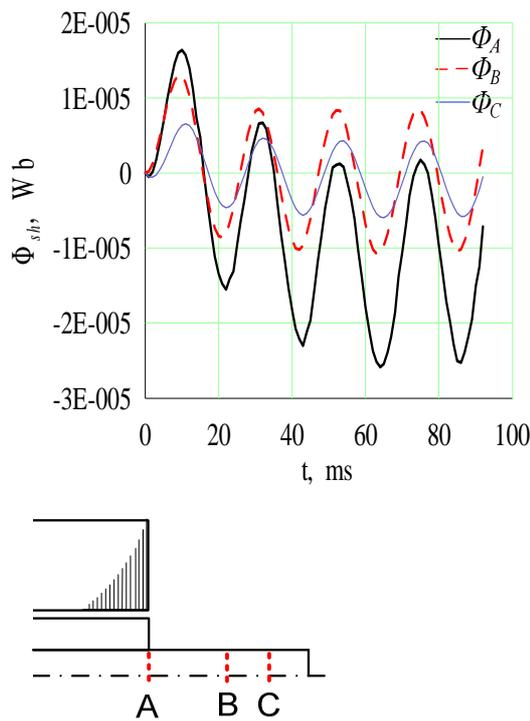
Fig. 5. Waveforms of shaft fluxes computed at the initial period of the start-up of the motor with uniform air-gap in the three shaft cross-sections A, B, C
