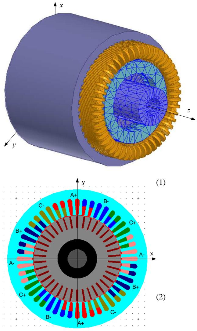
Fig. 2. Three-dimensional model of the induction motor and layout of the winding coils in the stator slots.
