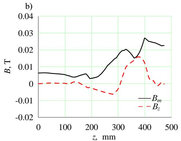
Fig. 4. Distribution of the magnitude  $B_m$  and the axial component  $B_z$  of the flux density in the air-gap (a) and in the shaft (b) in the plane passing through the axis of the shaft in the motor with uniform air-gap at the initial period of the start-up
