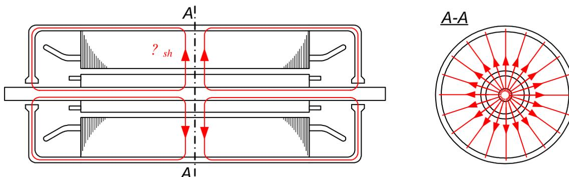
Fig. 1. Paths of homopolar fluxes in induction machine
