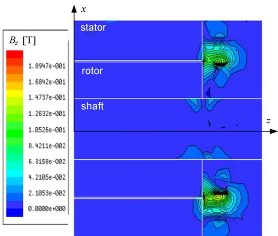
Fig. 3. Distribution of the radial (a) and axial (b) components of the flux density in the plane passing through the axis of the shaft in the motor with rotor eccentricity at the initial period of the start-up
