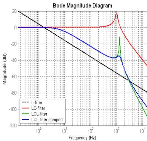
Fig. 7. Transfer functions of the filters
