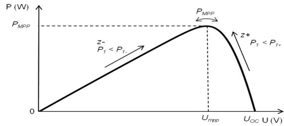
Fig. 3. MPP tracking principle
