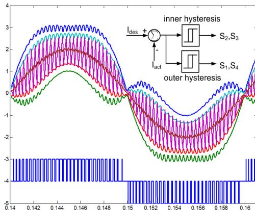
Fig. 5. Double hysteresis controller and its function
