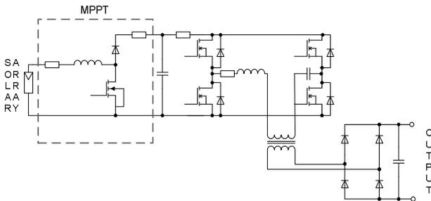
Fig. 2. DC/DC converter power part
