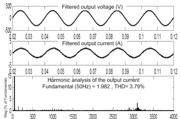
Fig. 8. Simulation of the designed filter influenc on the inverter
