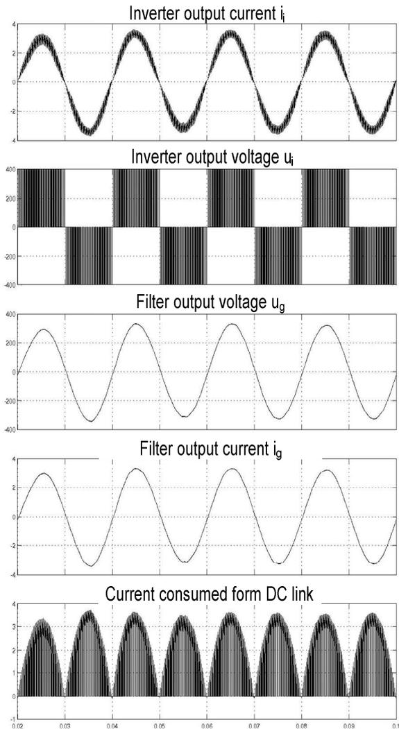
Fig. 10. Output of the converter – PWM control
