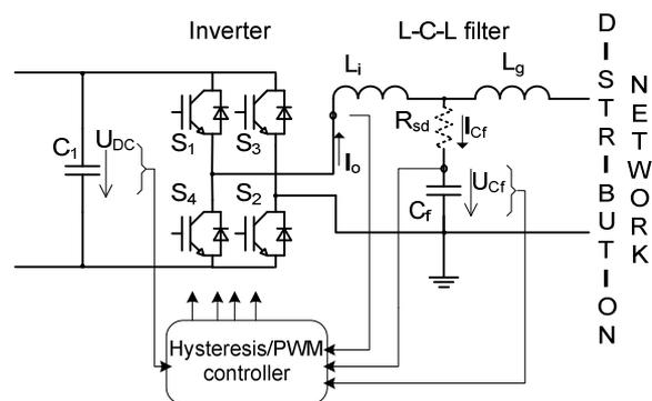
Fig. 4. Power part of the inverter
