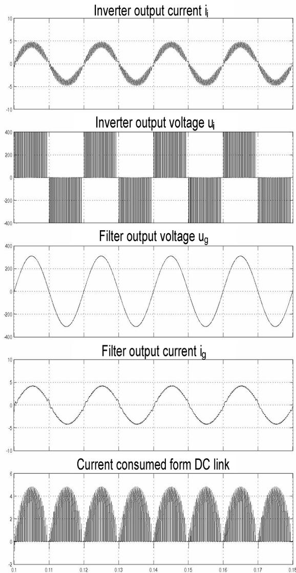
Fig. 9. Output of the converter - hysteresis control
