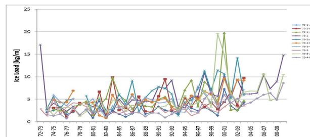
Figure 5. 39 years of ice loadings measured on 10 test spans in Iceland.
