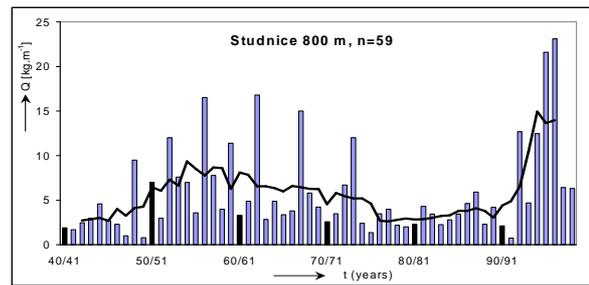
Figure 4. The longest continuous time series of ice load measurements in the world. Mt. Studnice, 800 m above sea-level, Czech Republic.
