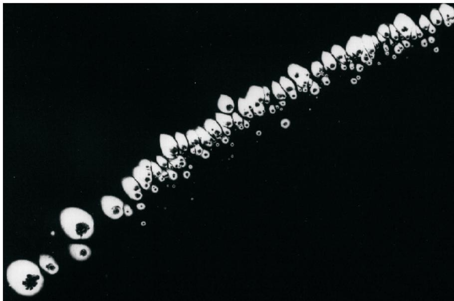
Fig. 1: Streamer spots on the dielectric barrier
