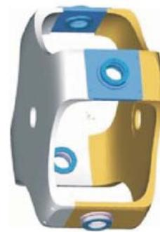
Fig. 7: The Stephenson-linkage housing made up of two identical covers
