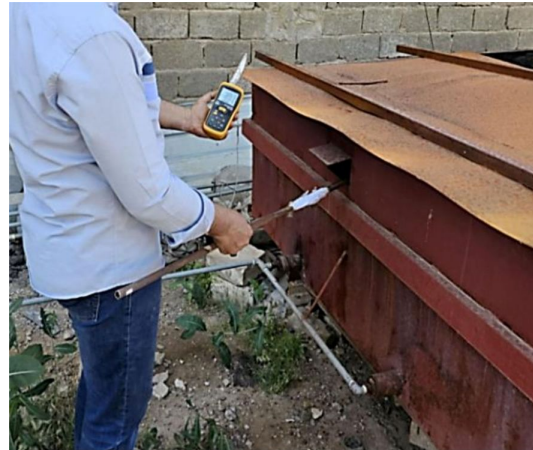
(B). Measuring temperatures with thermocoupling.
