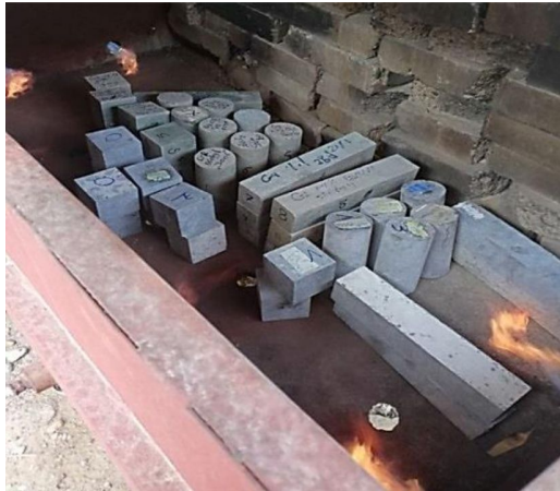
(A). Burning specimens by fire flame.
