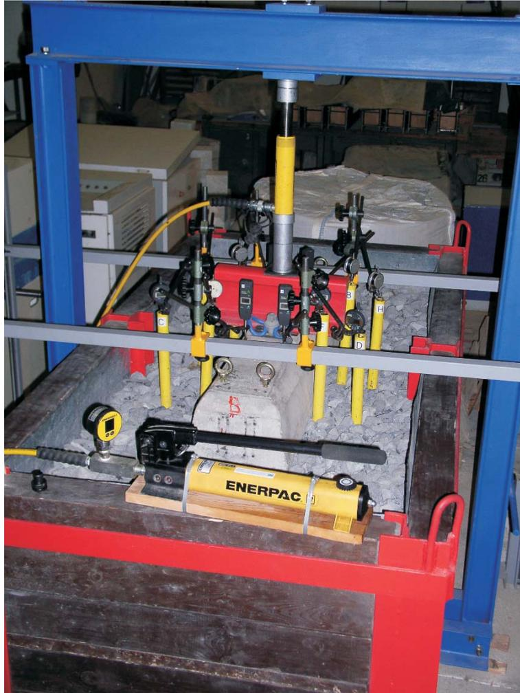
Fig. 6: Deflection measurement due to rail head load
