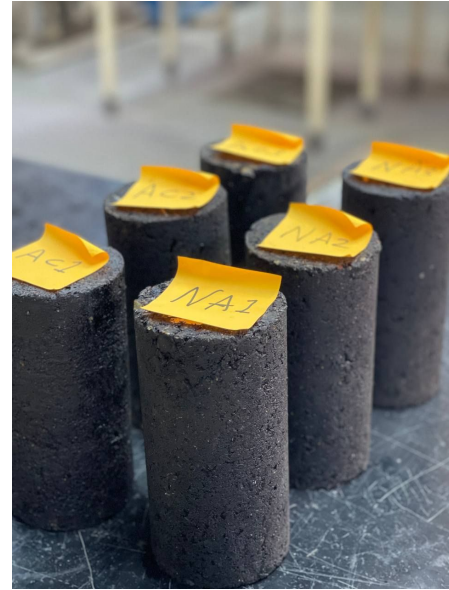
FIGURE 6. Group of specimens after mould extraction.
