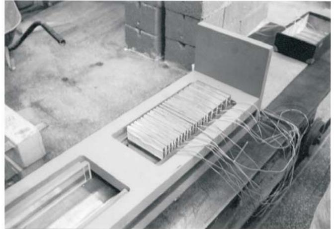
Photo 2: Loading cell. Right with sample and force meters.
