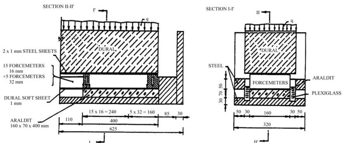
Fig. 1: Scheme of the loading cell
