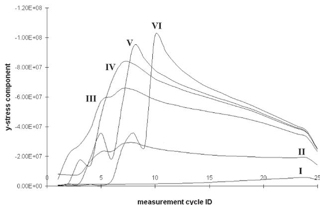
Fig. 9: Stress distribution along the coal seam
