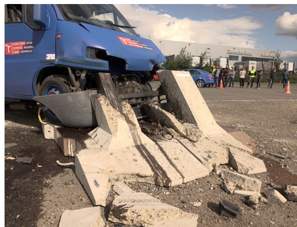
FIGURE 12. State after the vehicle stopped, second crash test. Note the bent interlocking bar in the front-left of the barrier.
