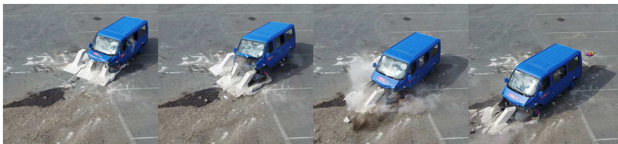
FIGURE 11. Progression of the crash test with the van.
