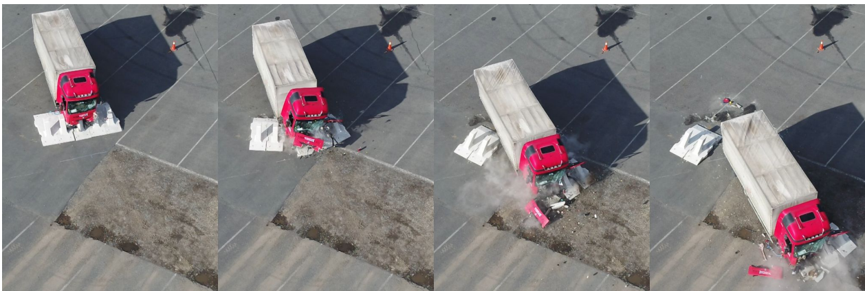
FIGURE 9. Progression of the crash test with the large goods vehicle.
