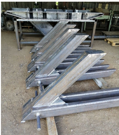
FIGURE 3. Welded steel profiles forming the barrier’s brace. In the back is the custom steel mould, note the upside-down orientation for casting concrete.
