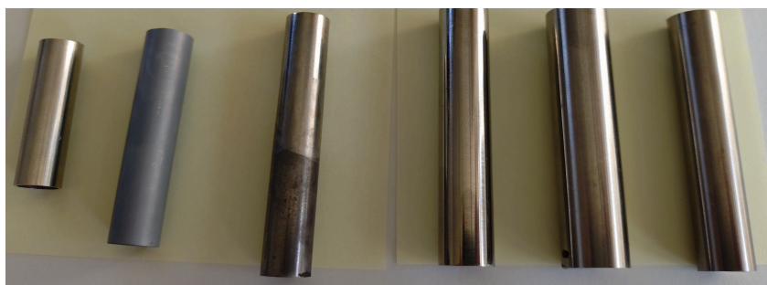
FIGURE 2. Samples used for tests (from left: CrNi alloy, matrix material with CrAl coating, reference sample Zr-1%Nb, FeCrAl old bar, FeCrAl new bar, FeCrAl new tube).
