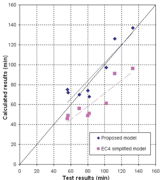
Fig. 4: Comparison of FRR, proposed numerical model, and EC4 model
