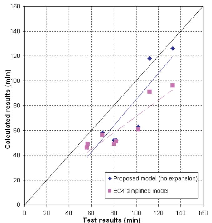
Fig. 5: Comparison of FRR, proposed model (without expansion), and EC4 model
