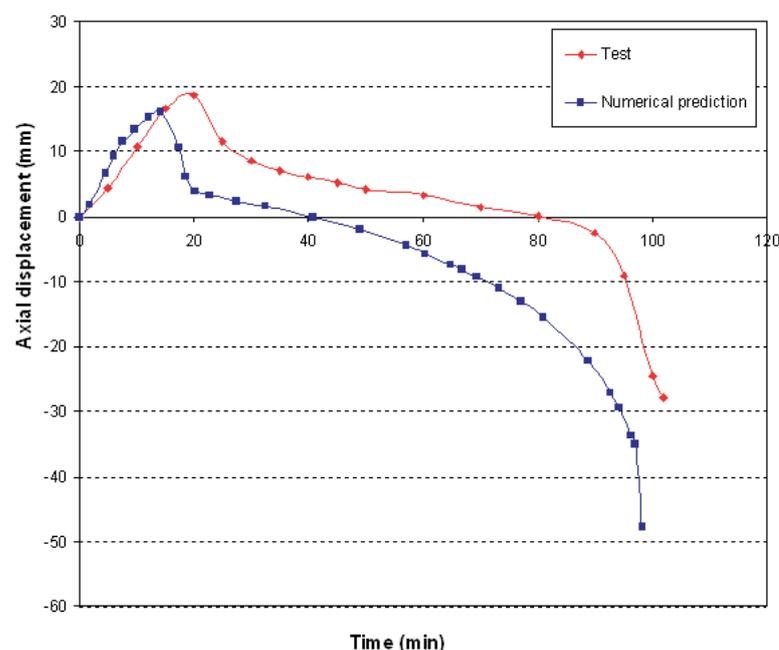
Fig. 1: Comparison between calculated and measured axial displacement, for test no. 4
