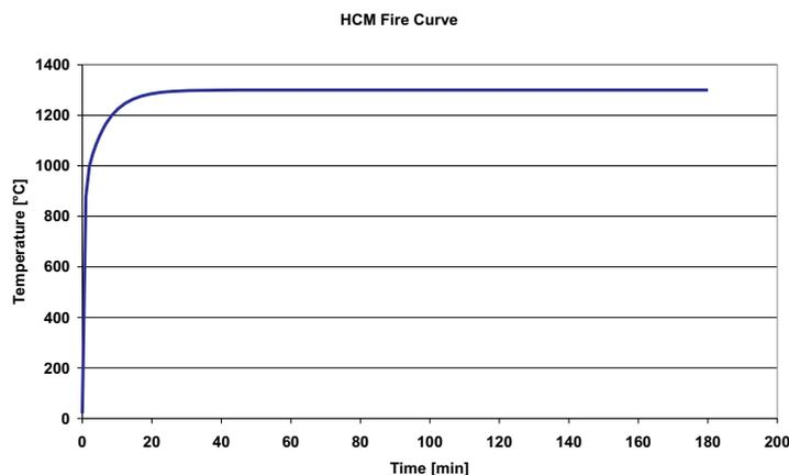
Fig. 15: Hydro Carbon Increased fire curve according to [7]
