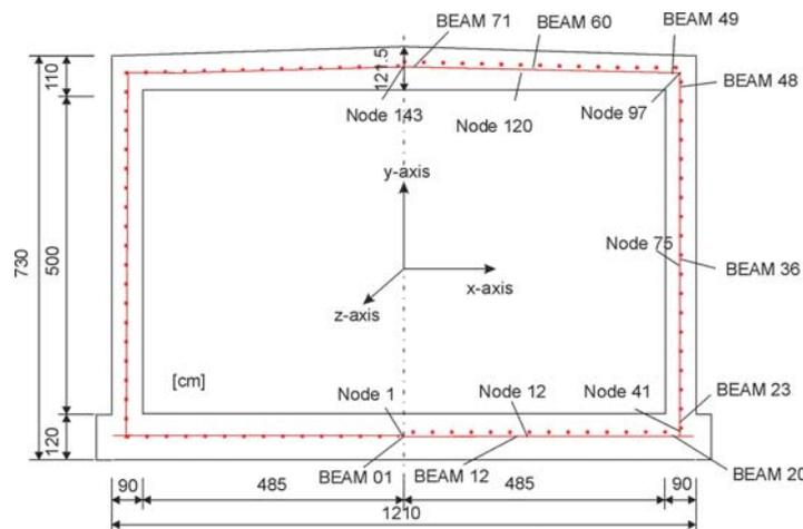
Fig. 14: Principle sketch of the tunnel; according to [22]
