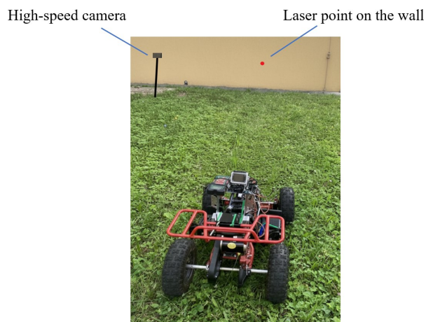
FIGURE 11. The position of the camera and the laser point on the wall.
