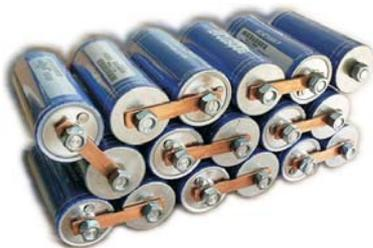
Fig. 1: Ultracapacitor battery pack
