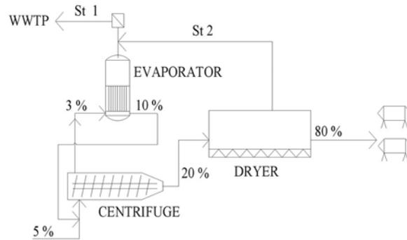
Fig. 1: Livestock feeding process line. Content of dry mass in wt. %
