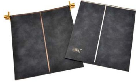
Fig. 2: The T-Resonator Structure
