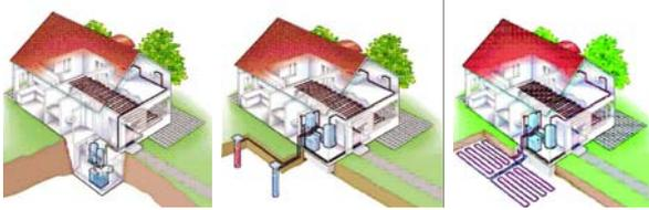
Fig. 2: Air, water, soil to water heat pumps [\*2]
