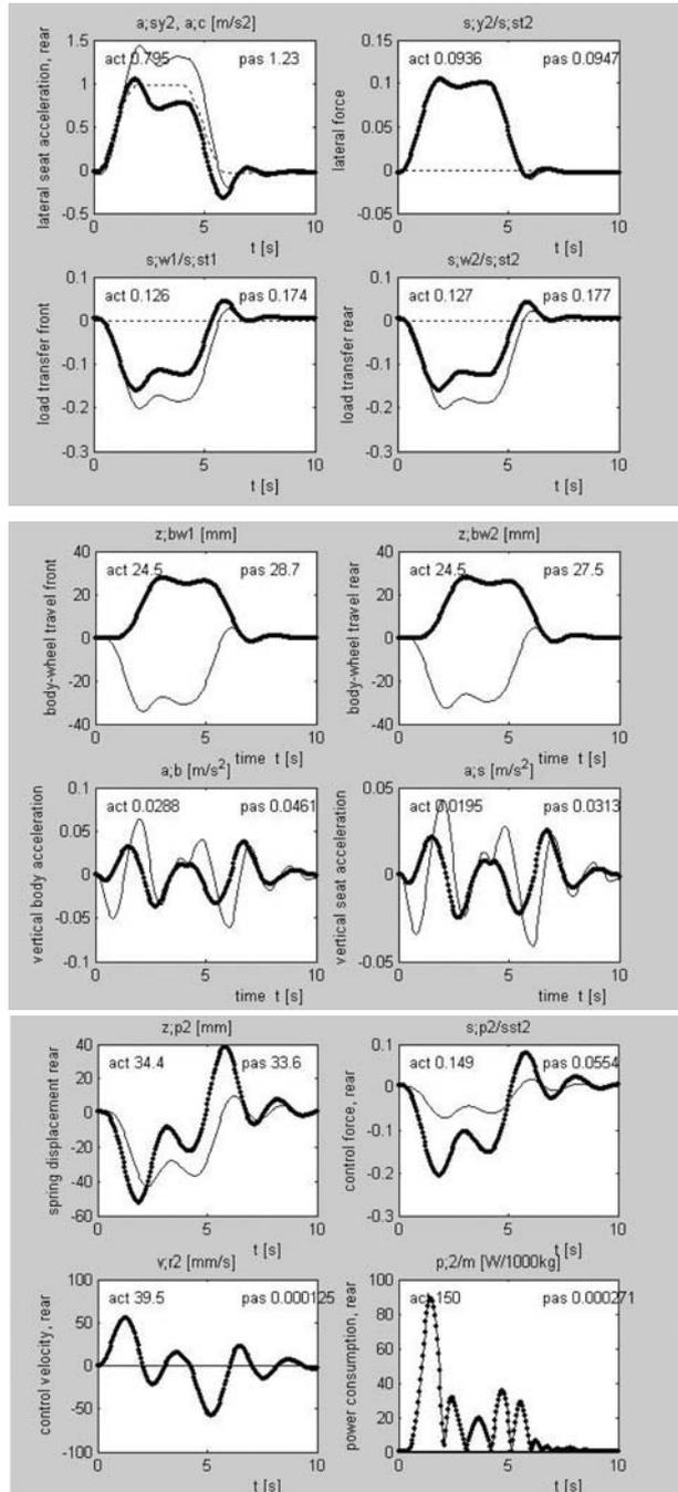
Fig. 4: Time histories due to the impulse of lateral acceleration. A thick line means an active variant (act), a thin line means a passive variant (pas). The attached numbers are imp-eff. values. A semicolon is used to mark an index. In the graph of power, the attached value refers to energy consumption [Ws/1000 kg]
