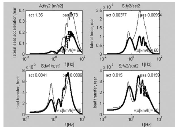
Fig. 5: Frequency characteristics due to unevenness. A thick line means an active variant (act), a thin line means a passive variant (pas). The attached numbers are imp-eff. values. A semicolon is used to mark an index
