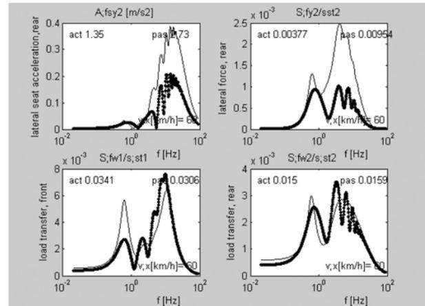
Fig. 5: Frequency characteristics due to unevenness. A thick line means an active variant (act), a thin line means a passive variant (pas). The attached numbers are imp-eff. values. A semicolon is used to mark an index
